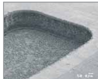
100 µm deep pockets in copper plated FR4
