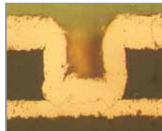
60 µm micro-via in RCC
