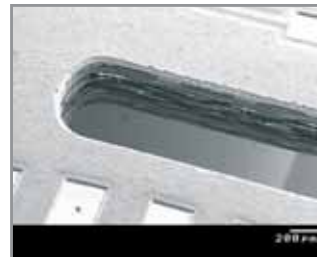
Inner contour cut in FR4-Multilayer
